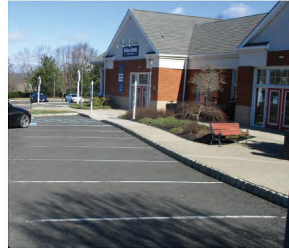
Parking spaces in the parking lot can be converted to porous pavement to capture and infiltrate stormwater runoff from the parking lot. Downspout planter boxes can be installed at the entrance of the building to beautify the space and capture stormwater runoff from the roof. A preliminary soil assessment suggests that more soil testing would be required before determining the soil's suitability for green infrastructure.
